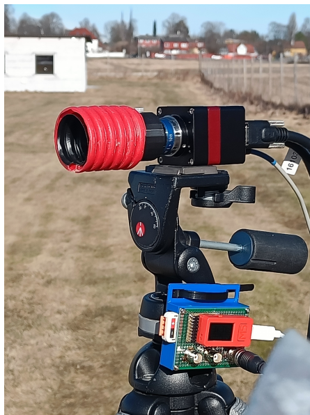
Figure 3.1.4: The camera that was used to conduct the experiments was the Raptor Photonics Owl 640S. The external triggering box is attached to the tripod below the camera.
