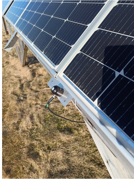
Figure 3.1.5: The Apogee pyranometer that was used is screwed right below the modules in order to capture the same irradiance as the modules.
