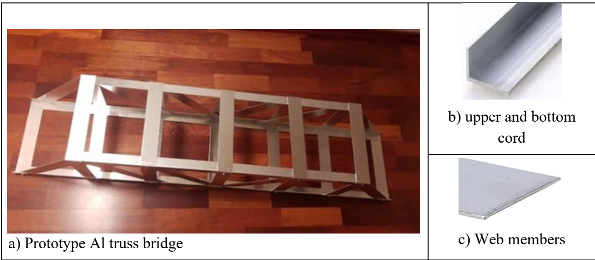
Figure 9: Pre -experimental model design 1500x250x250mm and its cross-sections
