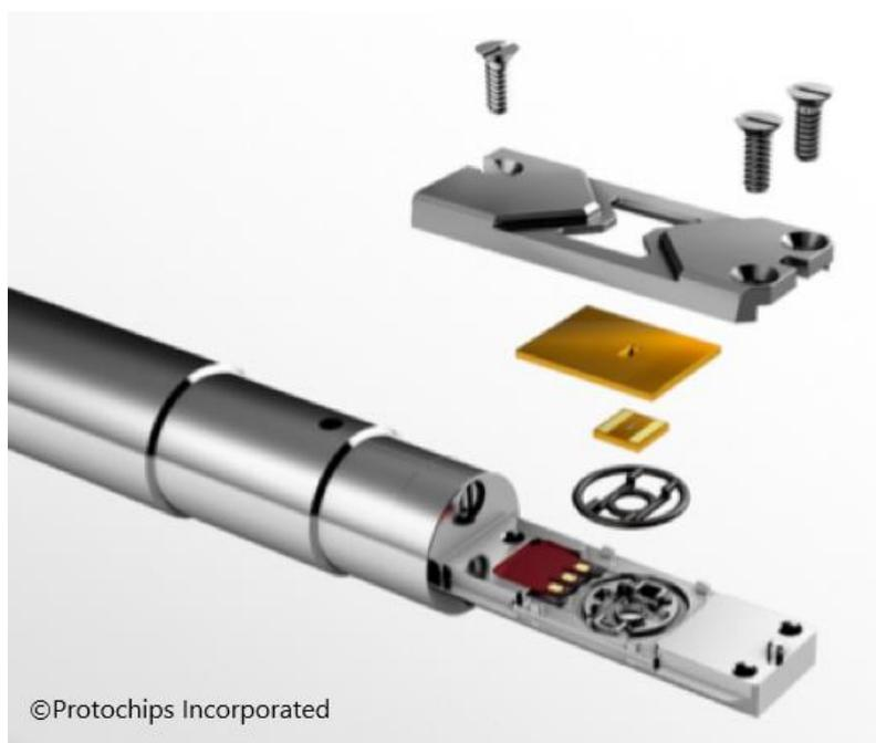
**Figure 1.6** The diagram of liquid-cell chip: Protochips Poseidon 300
