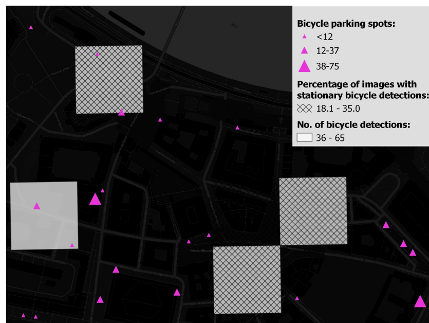
Figure 13. Example of visual analysis of bicycle parking capacity in Dresden by overlapping 100 \times 100 m grid cells of the N_{PB} (gray) and P_{PB} (hashed) layers in QGIS (version 3.16).
