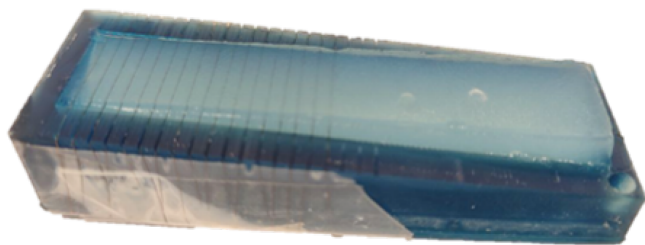
FIGURE 3 Photograph of the agar phantom inside the Three-dimensional (3D) printed mold. The human hairs inside the phantom are fixed with scotch tape and positioned at increasing depths with steps of 150\ \mu\text{m}
