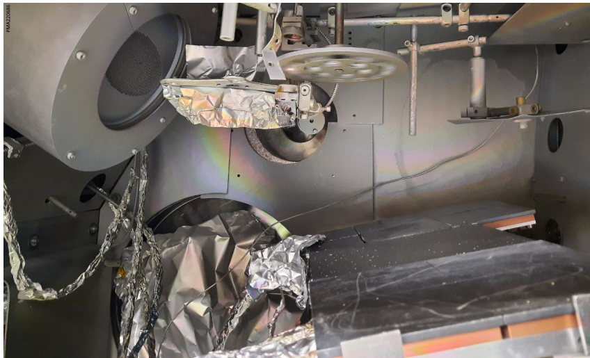
Figure 7.3: The coating machine used for the production of KBS. In the bottom right, the three target materials can be seen (arranged front to back). In the upper center, the rotating substrate carrier can be observed next to the ion source on the left.
