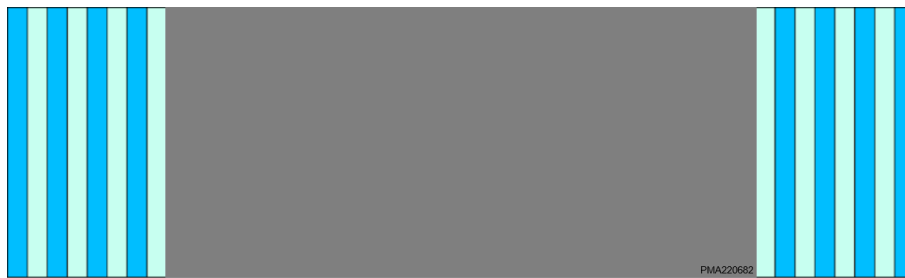
Figure 8.10: The schematic representation of a GaAs-KBS. Instead of a single coating on an optical substrate, a GaAs-wafer functions as the central spacer and the coating is deposited on both wafer surfaces.
