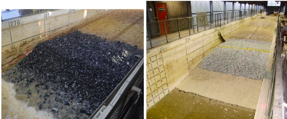
Fig. 1. (Left) The poorly-sorted revetment. (Right) The well-sorted revetment.
