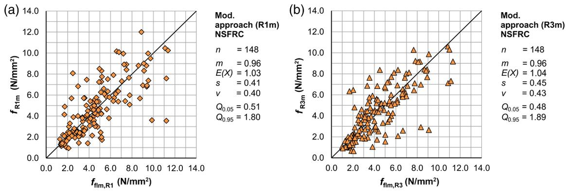
**FIGURE 9** Comparison of calculated residual flexural strength  $f_{flm,R1}$  and  $f_{flm,R3}$  with the mean value of the experimental residual flexural strength  $f_{R1m}$  (a) and  $f_{R3m}$  (b) using the modified approach for NSFRC. NSFRC, Normal-strength steel fiber-reinforced concrete
