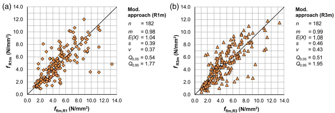
FIGURE 8 Comparison of calculated residual flexural strength  $f_{flm,R1}$  and  $f_{flm,R3}$  with the mean value of the experimental residual flexural strength  $f_{R1m}$  (a) and  $f_{R3m}$  (b) using the modified approach
