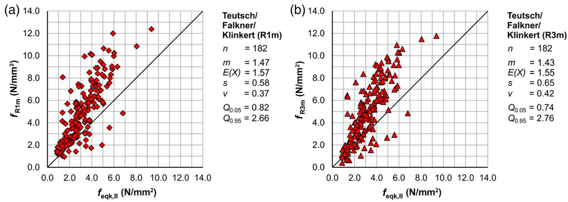
FIGURE 5 Comparison of calculated residual flexural strength  $f_{eqk,II}$  with the mean value of the experimental residual flexural strength  $f_{R1m}$  (a) and  $f_{R3m}$  (b) using the approach of Teutsch/Falkner/Klinkert<sup>16-18</sup>
