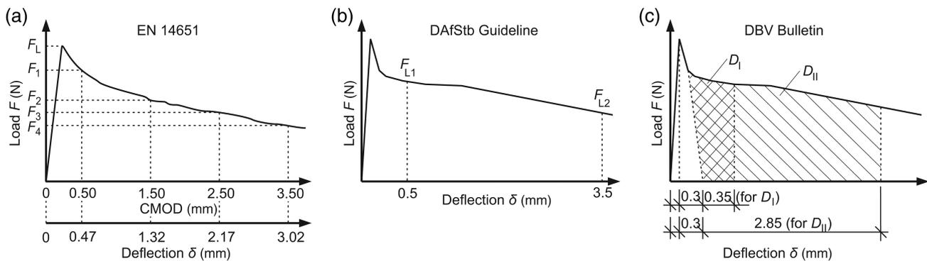
**FIGURE 1** Load–CMOD or load–displacement curve to determine the residual flexural tensile strengths according to DIN EN 14651<sup>5</sup> (a), the residual flexural tensile strengths according to DAfStb Guideline<sup>8</sup> (b), and the equivalent flexural tensile strengths according to DBV Bulletin<sup>12</sup> (c). CMOD, Crack mouth opening displacement
