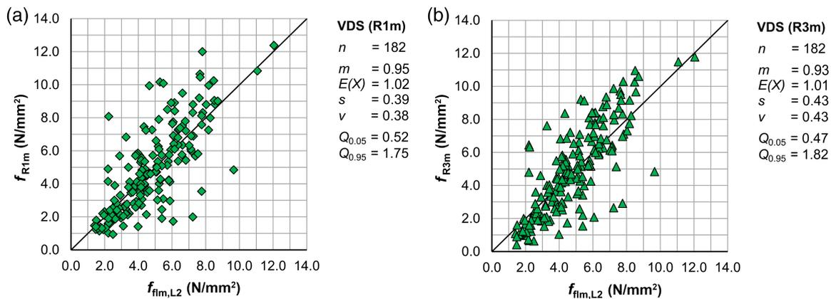
FIGURE 6 Comparison of calculated residual flexural strength  $f_{fim,L2}$  with the mean value of the experimental residual flexural strength  $f_{R1m}$  (a) and  $f_{R3m}$  (b) using the approach of VDS
