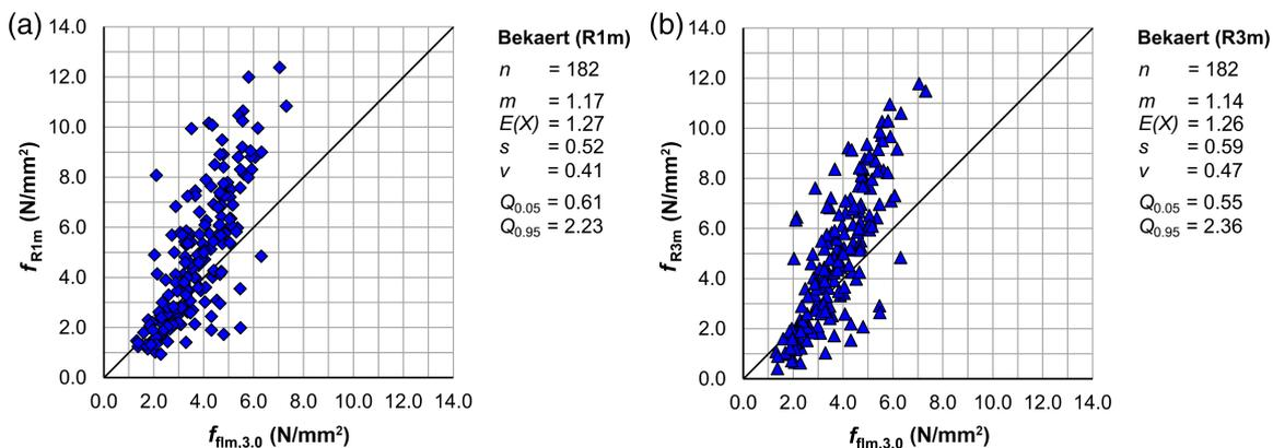
FIGURE 4 Comparison of calculated residual flexural strength  $f_{flm,3,0}$  with the mean value of the experimental residual flexural strength  $f_{R1m}$  (a) and  $f_{R3m}$  (b) using the approach of Bekaert<sup>15</sup>
