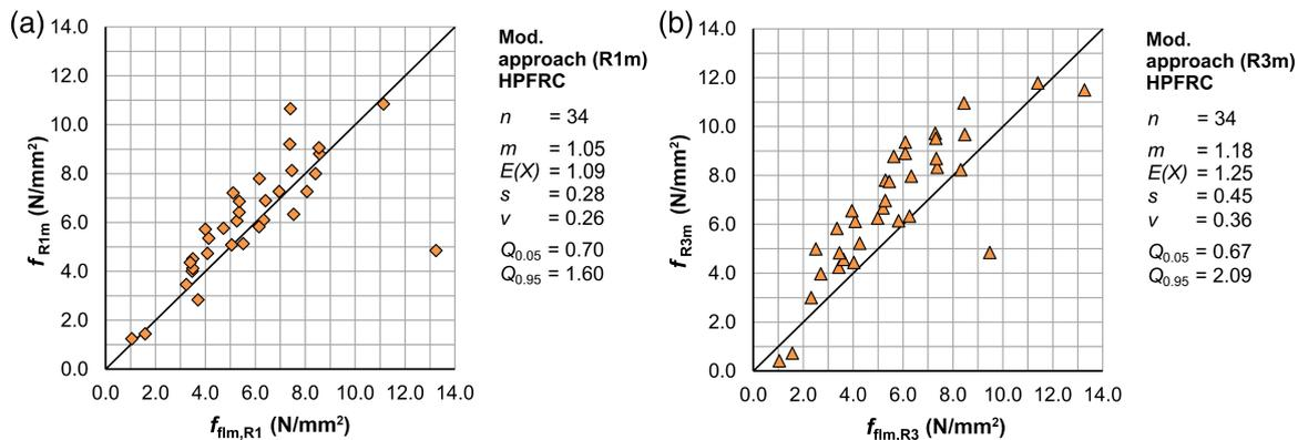
**FIGURE 10** Comparison of calculated residual flexural strength  $f_{flm,R1}$  and  $f_{flm,R3}$  with the mean value of the experimental residual flexural strength  $f_{R1m}$  (a) and  $f_{R3m}$  (b) using the modified approach for HPFRC. HPFRC, High-performance steel fiber-reinforced concrete
