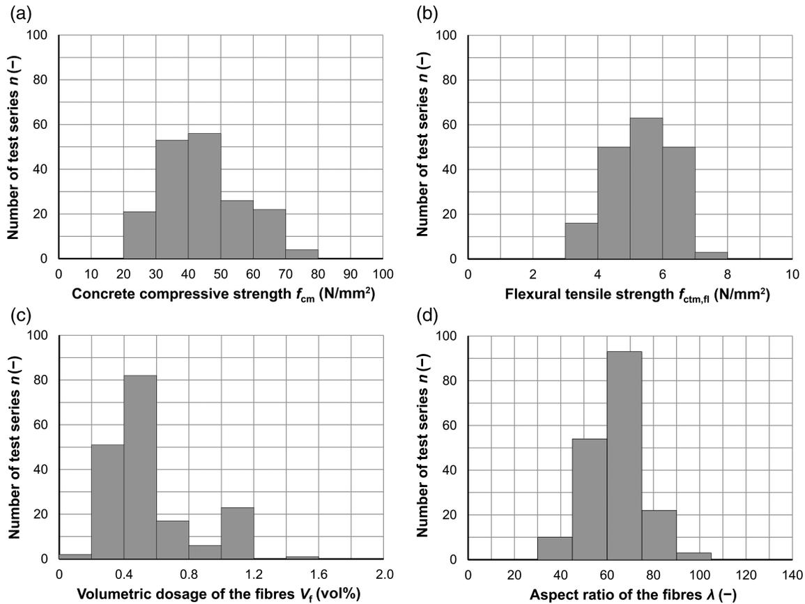
**FIGURE 2** Range of parameters of the used data with regard to (a) concrete compressive strength  $f_{cm}$ , (b) flexural tensile strength of the concrete  $f_{ctm,fl}$ , (c) volumetric dosage of the fibers  $V_f$ , and (d) aspect ratio of the fibers  $\lambda$
