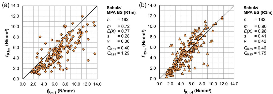
FIGURE 7 Comparison of calculated residual flexural strength  $f_{Rm,1}$  and  $f_{Rm,4}$  with the mean value of the experimental residual flexural strength  $f_{R1m}$  (a) and  $f_{R3m}$  (b) using the approach of Schulz/MPA BS
