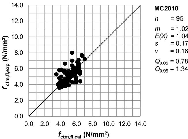
FIGURE 3 Comparison of calculated flexural tensile strength  $f_{ctm,fl}$  according to MC2010 with the experimental flexural tensile strength  $f_{ctm,fl,exp}$
