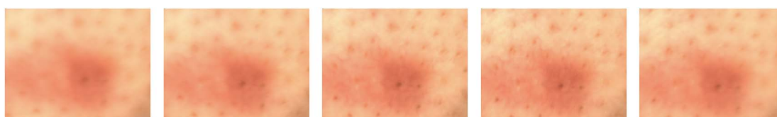
Figure 9. Captured input images for different currents of the liquid lens (liquid lens current from left to right image: 103 mA, 109 mA, 115 mA, 121 mA, 127 mA).
