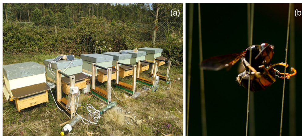
Figure 1. Protection system: six hives placed in line, separated 20–30 cm each, protected with five electric harps (a). When hunting honey bees in front of the hives, hornets fly between electrified wires that paralyze them (b). Afterwards they fall into a cage from which smaller insects escape while hornets fall into a collection bottle.
