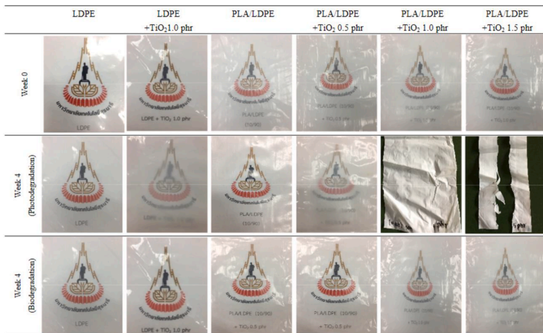
Fig. 5. Appearance of LDPE films in which 10 wt.% PLA or both 10 wt.% PLA and different amounts of TiO 2 have been added. The samples were imaged at week 0 and then at week 4 of irradiation with sunlight and at week 4 after biodegradation experiments. Reprinted from [13], copyright (2019), with permission from Elsevier.
