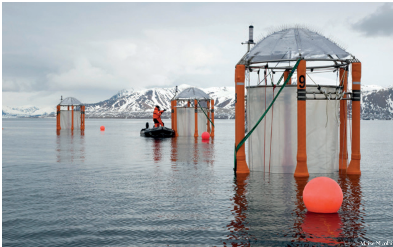
Scientists sampling mesocosms during an outdoor experiment investigating the reactions of marine organisms to ocean acidification at Kongsfjord, Ny-Alesund, Svalbard.
