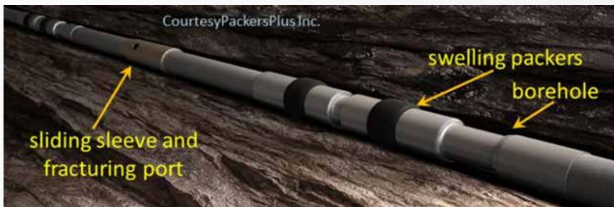
Figure E.2 The Sliding Sleeve and Ball Method for Shale Gas Well Completion
