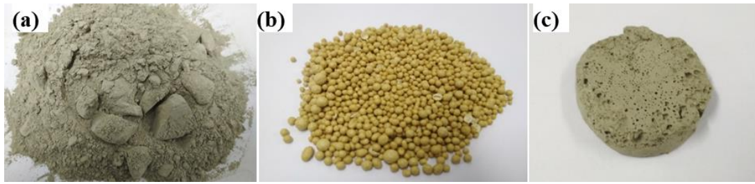
Fig. 1 – Raw materials and prepared porous fly ash bricks; (a) Coal fly ash powder, (b) baking yeast, (c) Porous fly ash brick sample Equations
