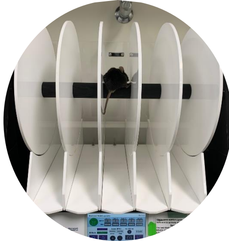
Figure 6-5: Configuration of the Rotarod device. During the test, the mice were separated into five lanes, as seen in the image, and their latency is automatically recorded using individual levers.
