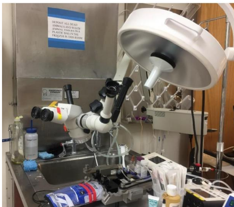
Figure 6-1: Surgery table setup for performing craniectomy surgeries on mice.
