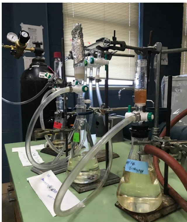
Figure 3-1: Illustration of N-terminus peptide synthesis using solid phase peptide vessel under inert atmosphere.
