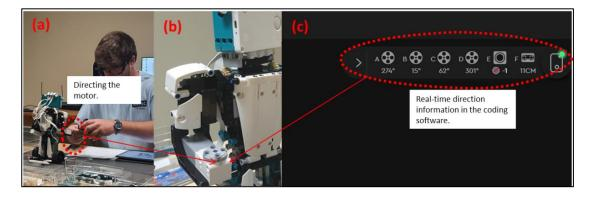
**Figure 6-7:** Manual assembly of the robot's claw. (a) Assembler directing the motor in the specified degrees. (b) Enlarged view of the arm's motor in the zero direction. (c) Real-time positioning data which the assembler monitors simultaneously in Mindstorms® software.
