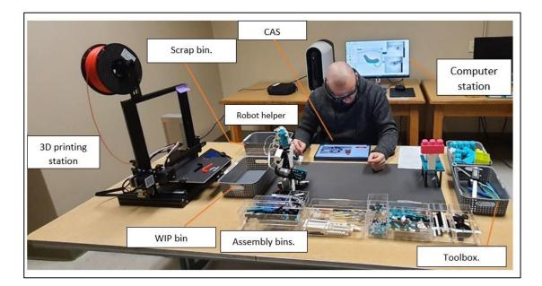
**Figure 6-6:** Experiment 2 workstations: the assembly workstation, the PC workstation, the 3D printing workstation, and the robot workstation.
