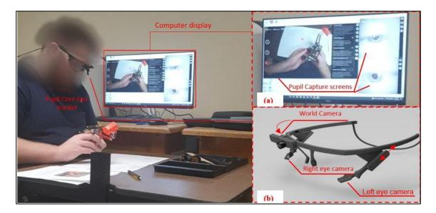
**Figure 4-1:** (Left) Experimental apparatus. (Right) (a) Pupil Capture desktop app real-time display of the experiment captured by the eye tracker cameras (b) Pupil Core eye tracker.
