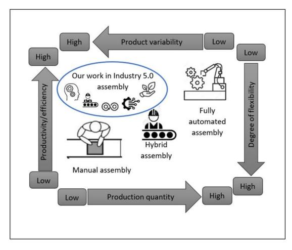
**Figure 6-2:** Manual assembly, hybrid assembly, fully automated assembly, and our research elements in the Industry 5.0 work environment (based on "Changeable and Reconfigurable Assembly Systems by B. Lotter and H.-P. Wiendahl (2009)") [61].
