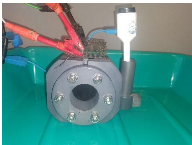
Figure 3. General view of the specially designed three-electrode unit cell
