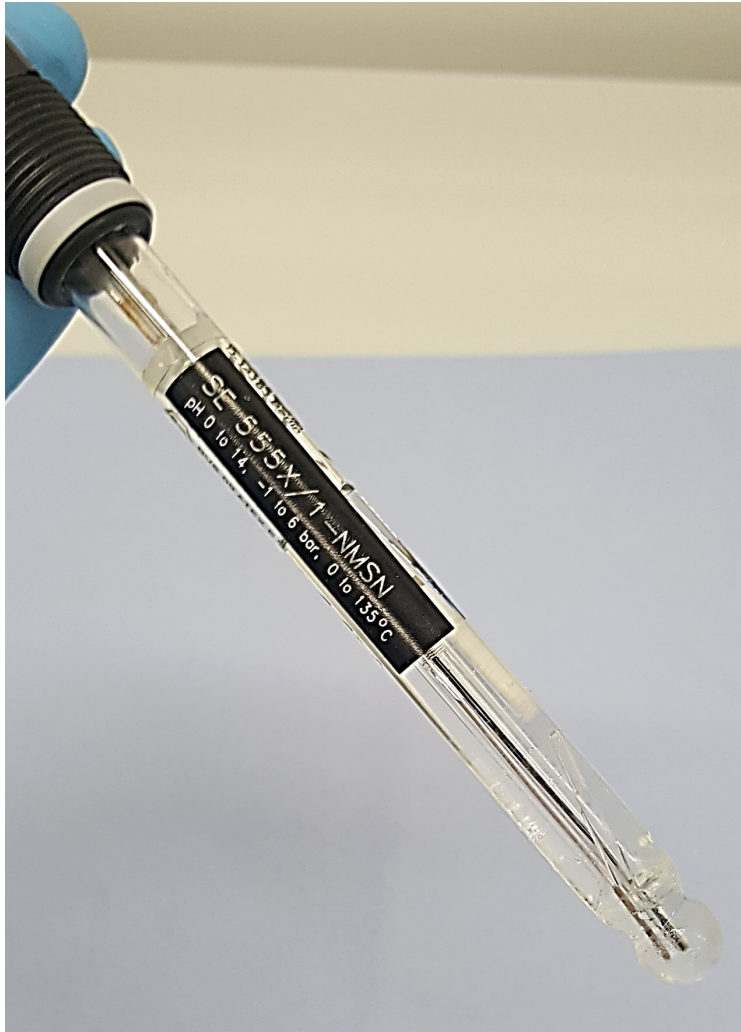
FIGURE 5.4: Inline pH sensor.
