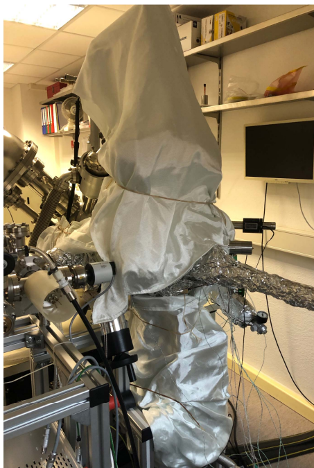
Fig. 37 Photo of the preparation chamber during the bake-out procedure, wrapped with bake-out cables, layers of Al foil, and glass fiber cloths to achieve UHV conditions.
