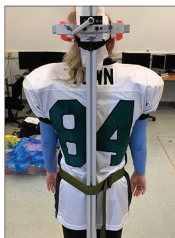
Figure 1. Stabilizing apparatus with hip strap and adjustable head stabilization device
