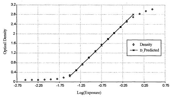
Figure 8, Hurter-Driffield Curve For KODAK 3034 Film, with fitted line to the linear region
