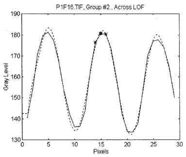
Figure 12, Mean Lateral Cross-Section Plot of Bar Group #2 and 10<sup>th</sup> Order Polynomial Fit (Solid Line: Bar Group Data; Dashed Line: 10<sup>th</sup> Order Polynomial Fit; Markers: the centroid and adjacent points)
