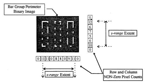
Figure 25, Demonstration of x-range and y-range extent determination
