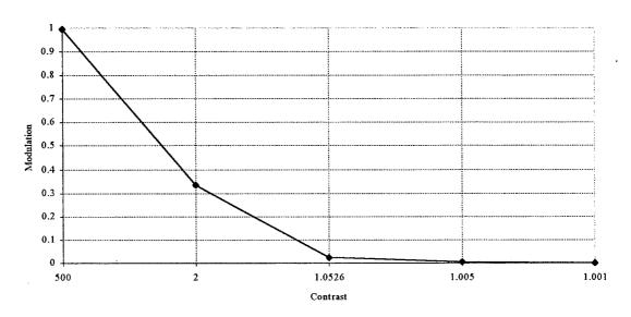
Figure 7, Comparison of Modulation and Contrast for a Fixed Exposure Difference of 500 µJ
