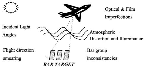
Figure 5, Sources of GRD Degradation<sup>10</sup>
