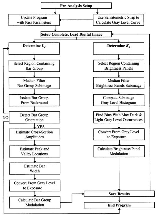
Figure 21, Flowchart of Adaptive Digital Method
