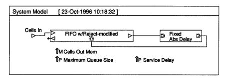
Figure 19 Block diagram of network model, or in this case a single link to an ATM network.
