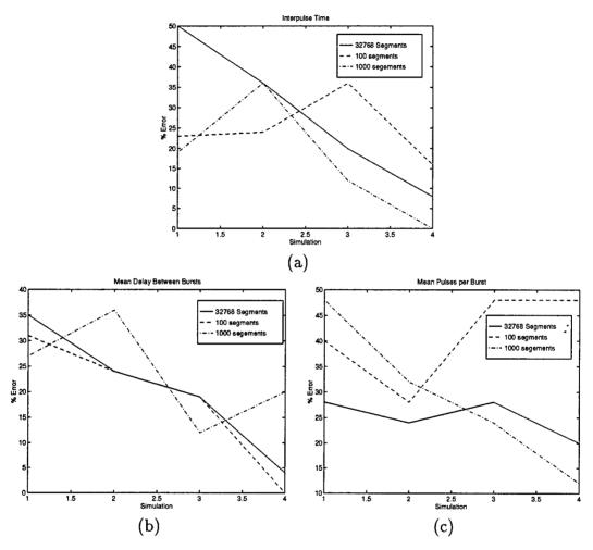
Figure 6 Segmentation scheme error for each of three parameter set subgroups (a) IPT (b) MDBB and (c) MPPB. Plots show the 32,768 segment scheme has the most consistently decreasing error rate as parameter sets are moved away from the boundary.
