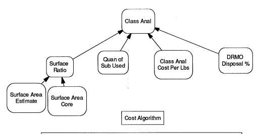
Class Analysis = Surface Ratio\*Quantity Substance Used\*Class Analysis Cost
