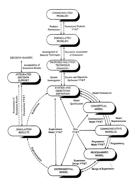
Figure 2.1 Balci's simulation study schematic (Balci, 1994:154)
