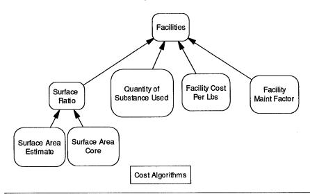
Facilities = (Surface Ratio\* Quantity Substance Used\*Facility Cost)\*(1+Facility Maint Factor)
