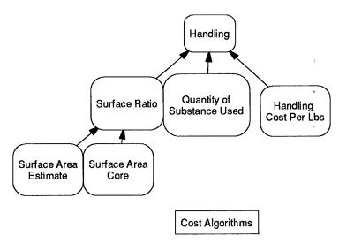
Handling = Surface Ratio x Quantity Substance Used x HandlingCost Factor
