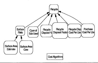
Recycle = Surface Patio\*Quantity Substance Used\*Recycle Disposal Percent\*Recycle Disposal Factor\*(Recycle Disposal Cost-Purchase Cost)
