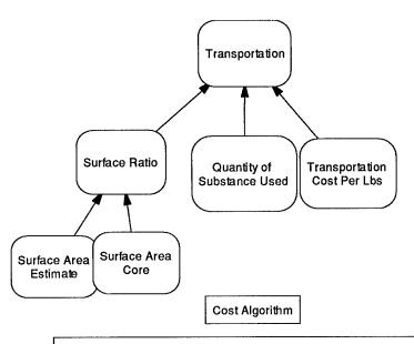
Transportation = Surface Ratio\*Quantity Substance Used\*TransCost
