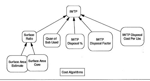
IWTP = Surface Ratio\*Quantity Substance Used\*IWTP Disposal Percent\*IWTP Disposal Factor\*IWTP Disposal Cost
