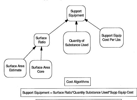
Surface Ratio = Surface Area Estimate/Surface Area Core
