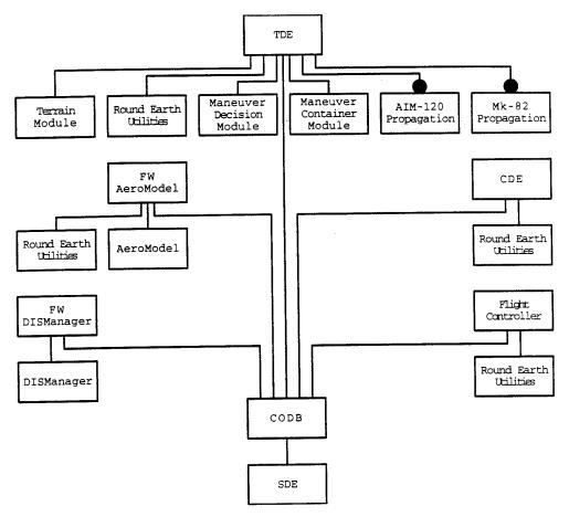
Figure 6.1. Object diagram of the Fuzzy Wingman.
