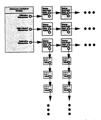
Figure 6.9. Organization of maneuvers within the Maneuver Container Module.
