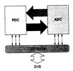
Figure 4.2. CGF architecture showing the Physical Dynamics Component, Active Decisions Component, and CGF Router.
