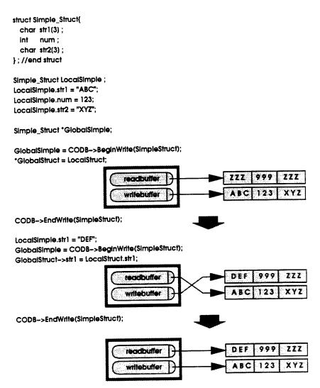
Figure 6.3. The stale data persistence phenomenon. If the contents of readbuffer aren't copied over to writebuffer before writing only portions of the structure, then stale data will persist in the unwritten portions.
