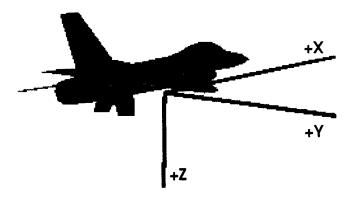
Figure 6.4. The Aircraft Body Coordinate System.
