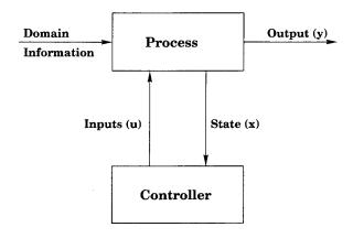
Figure 7.1 Fundamental closed-loop controller
