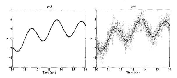
Figure 5.3. Plant Output with Representative High Noise Levels
