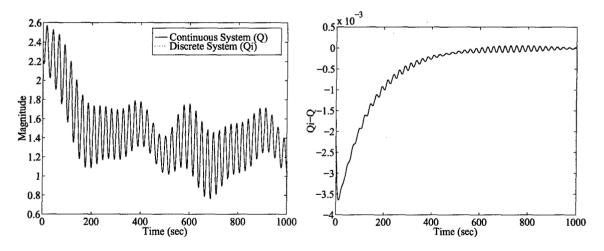
Figure 6.2. Comparison of Continuous and Discrete Outputs
