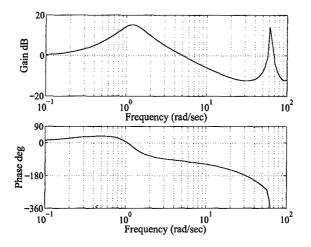
Figure 5.1. Discrete Bode Plot of Given Plant
