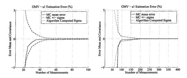
Figure 5.20. Incremental  $a_1$  Estimation for 0.1 (left) and 0.025 (right) Sampling Times
