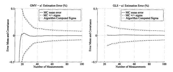
Figure 5.8. Incremental  $a_1$  Estimation for p = 3 without Initial Time
