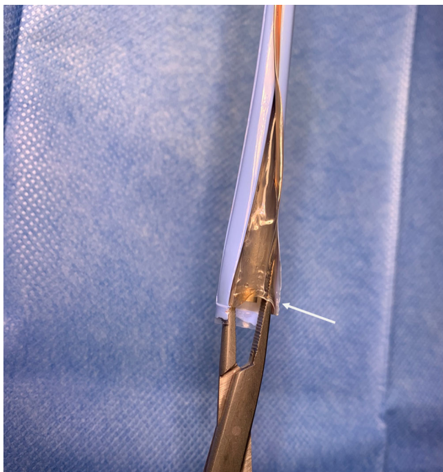
FIGURE 7 Used 14F eSheath after an uncomplicated case with a 23-mm Sapien 3 Ultra. A gap is evident between the inner and outer coats (arrow). [Color figure can be viewed at wileyonlinelibrary.com ]
