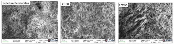
Fig. 9 - SEM images for samples before and after stabilization
