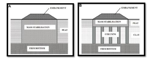
Fig. 2 - (a) Mass stabilization method; (b) combination of mass and column stabilization methods
