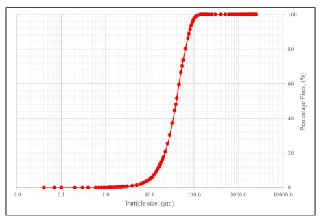
Fig. 8 - Particle size distribution graph for SCBA material
