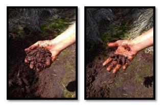
Fig. 1 - Von Posttest during soil sampling
