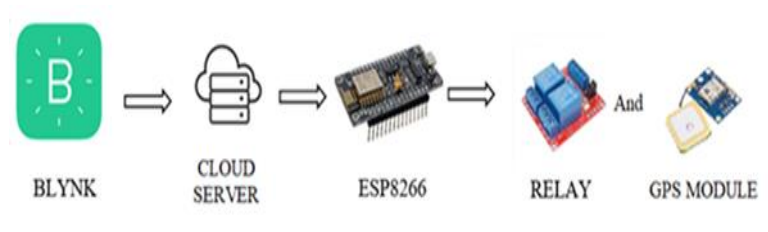
Fig. 2 - Blynk system with hardware
