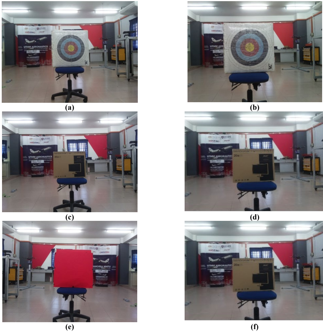
Fig. 7 - Captured image of the texture-less obstacle at (a) 150 cm; (b) 120 cm, semi texture obstacle at; (c) 150 cm; (d) 120 cm, texture-less obstacle at; (e) 150 cm; (f) 120cm
