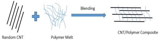
Fig. 8 - Steps in Melt mixing of CNT/Polymer Composite. Figure adapted from [74]
