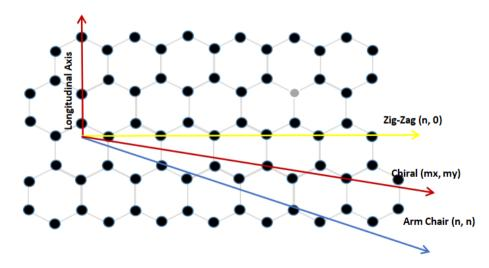
Fig. 2 - Single-walled carbon nanotubes configurations. Figure adapted from [24]
