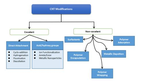
Fig. 7 - Approaches to CNT modification via functionalization. Figure adapted from [61-63]
