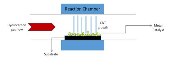
Fig. 6 - Chemical vapor deposition synthesis of Carbon Nanotubes. Figure adapted from [41]
