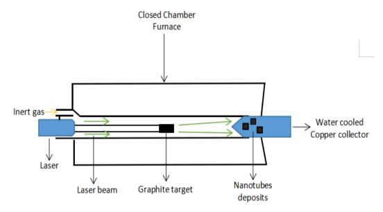
Fig. 4 - Oven laser-vaporization apparatus. Figure adapted from [33]
