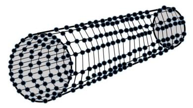
Fig. 1 - Single-walled carbon nanotubes. Figure adapted from [24]
