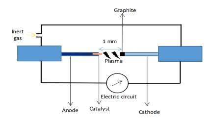
Fig. 5 - Electric arc discharge synthesis of Carbon Nanotubes. Figure adapted from [34, 35]
