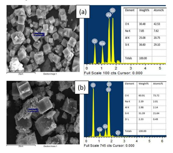
Fig. 3 - SEM and EDX result of the synthesized zeolite for (a) sample using turmeric plant extract; (b) sample using ginger extract
