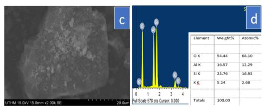
Fig. 1 - SEM image and EDX spectra for (a-b) kaolin (c-d) metakaolin
