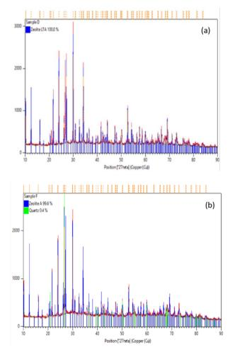
Fig. 2 - XRD Diffractogram of the synthesized product (a) sample using turmeric plant extract (b) sample using ginger plant extract
