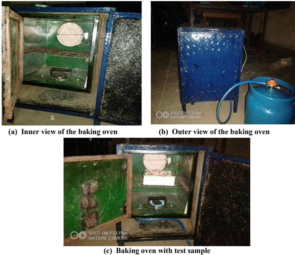
Fig. 4 - Constructed dual-powered baking oven
