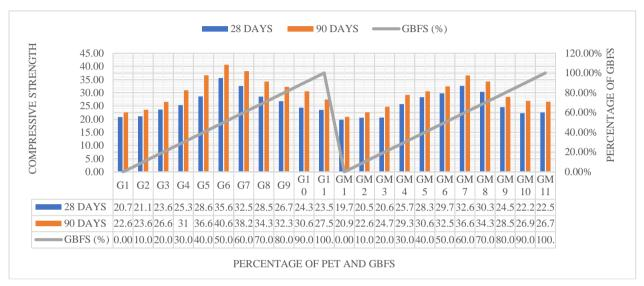
Fig. 8 - Compressive strength of samples with PET and GBFS [64]
