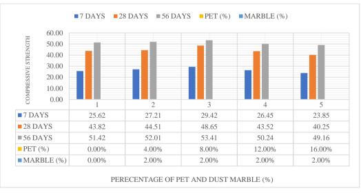
Fig. 7 - Compressive strength of samples with PET and dust marble
