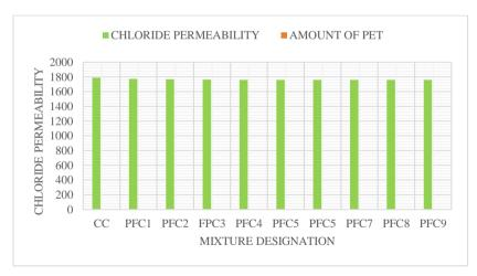
Fig. 5 - Chloride permeability reading for the sample mixes with plastic [59]
