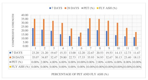
Fig. 6 - Compressive strength of samples with PET and fly ash [62]
