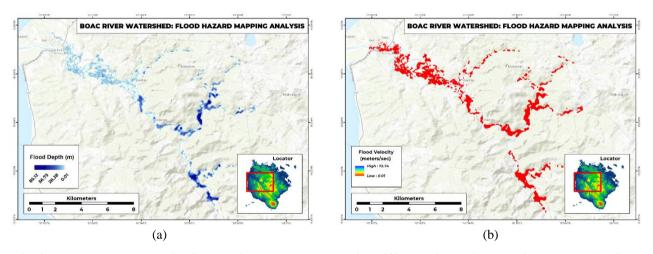
Fig. 3 - Flood hazard analysis of Boac River watershed showing different simulations; (a) flood depth; (b) flood velocity
