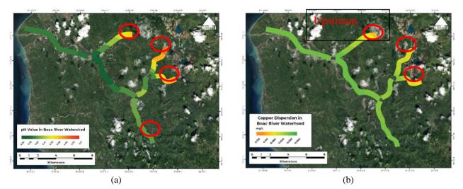
Fig. 4 - Spatial variability maps for water parameters of Boac River, Marinduque; (a) pH levels; (b) Cu dispersion
