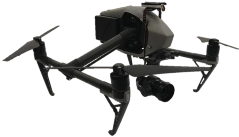
Figure 3.2: DJI Inspire II quadcopter with Zenmuse X5s sensor and DJI MFT 15mm lens.
