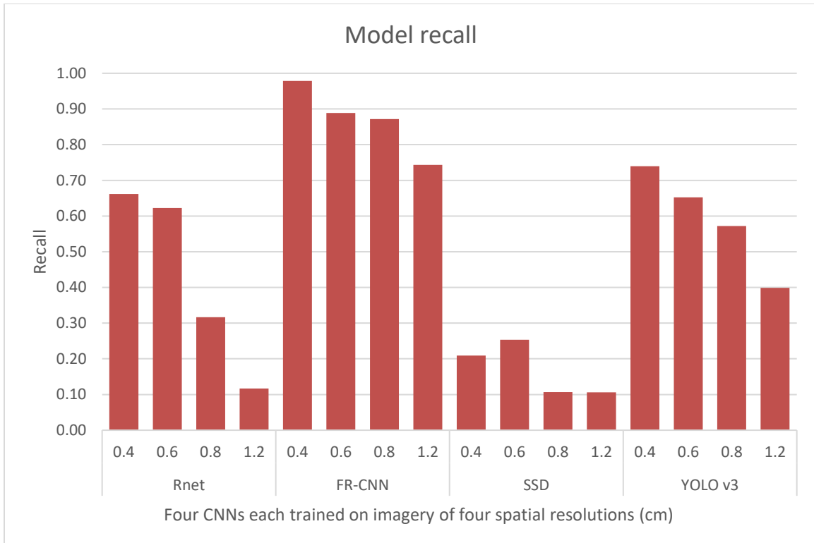
Figure 3.22: Recall results of 16 models evaluated on imagery from four production fields with 7,800 weeds.
