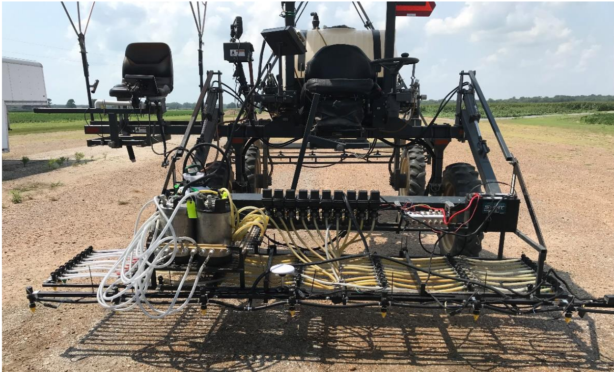
Figure 4.7: Site-specific Boom mounted on high-clearance sprayer.
