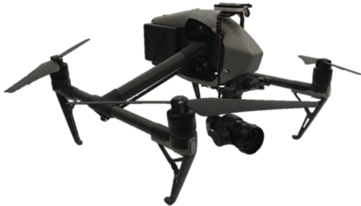
Figure 4.3: DJI Inspire II and Zenmuse X5s (iFlight Tech Company Ltd. Shenzhen, China) UAS used to collect plot imagery.
