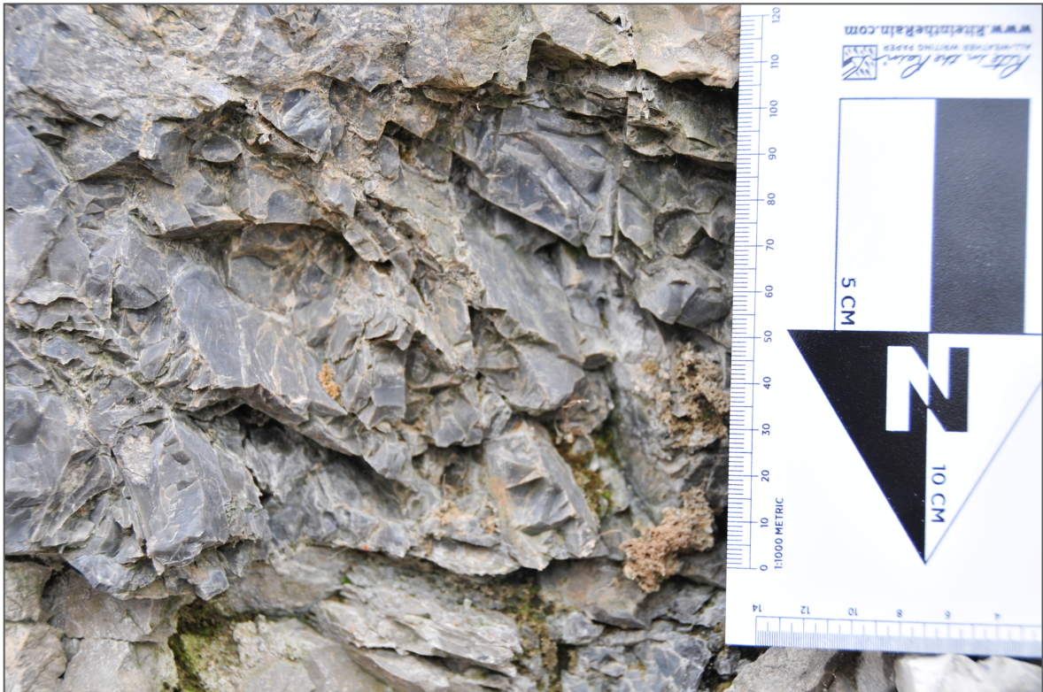
Figure 8. Shrinkage fractures in lower Boone chert. Photo by author.
