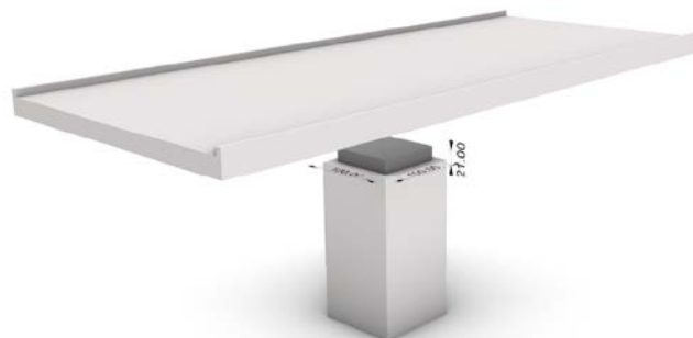
Figure 15. Suggested arrangement for the pentamode bearing
