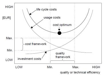
Figure 1. Cost optimum quality and technical efficiency (own representation based on [10])
