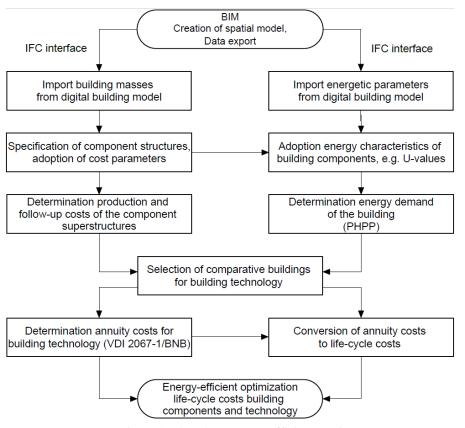
Figure 3. Flowchart energy-efficient costing
