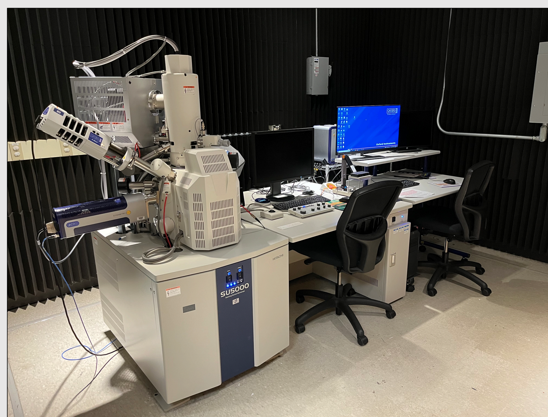
Figure 4: Hitachi SU5000 Scanning Electron Microscope (SEM)
