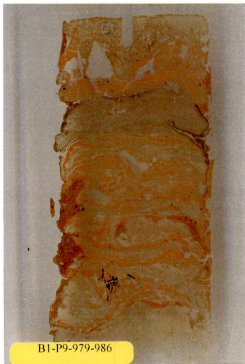
979-986 cm depth, Soil horizon Cr2 Gravelly silty clay. Note the horizontal relict bedding of deeply weathered shale and siltstone lithorelicts. Deeply weathered plant material / root traces. RF include coarse-equant dolostone and oolitic/pelloidal dolostone.
