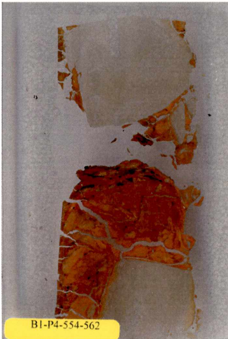
554-562 cm depth, Soil Horizon Bt4, clay Well-developed, Fe-rich pedogenic clay coatings. Note weathering rim around perimeter of dolostone fragments.
