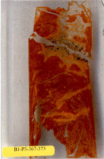
367-373 cm depth, Soil Horizon Bt1, silty clay Possible loamy infilling within root pore, pedogenic clay coloration and mottling clearly showing active macropores.
