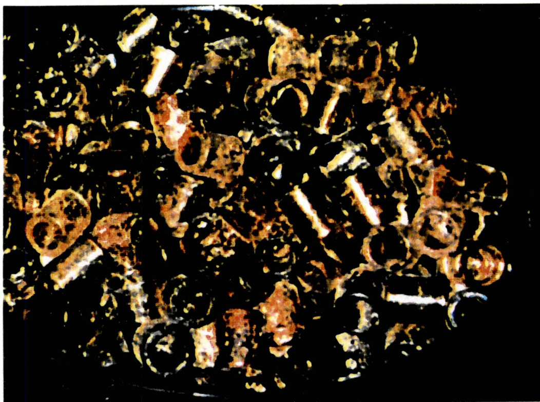
Figure 3.2 Radioactively contaminated borosilicate Raschig rings with thin dry film of contamination.
