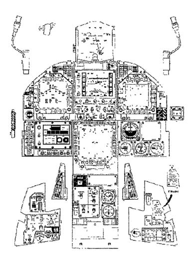
Figure A-1 Cockpit Layout of the F/A-18
