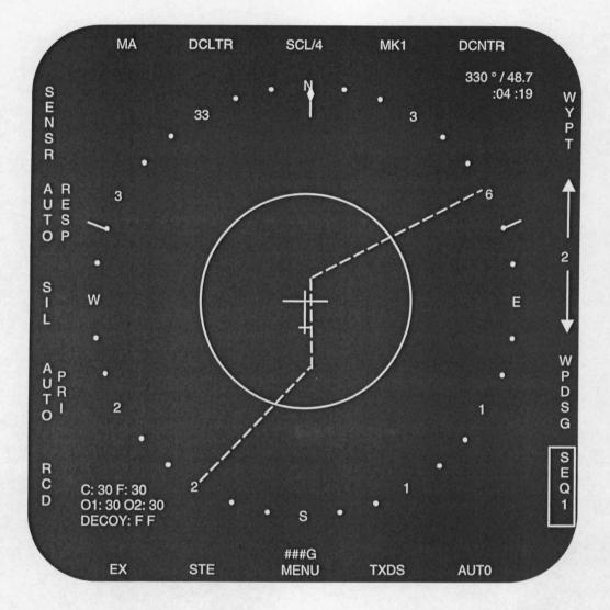
Figure 3-1 Navigation features of the combined SA format
