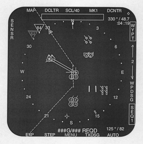
Figure 3-4 Data Link Trackfiles on the SA format
