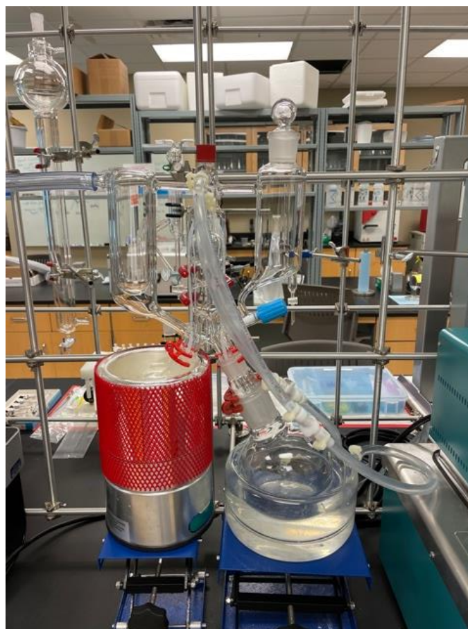
Figure 7 Solvent Assisted Flavor Evaporation (SAFE) apparatus
