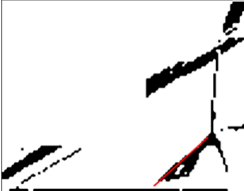
(a) Threshold-bounded Binarized Image w/ Shock Tracker Overlay
