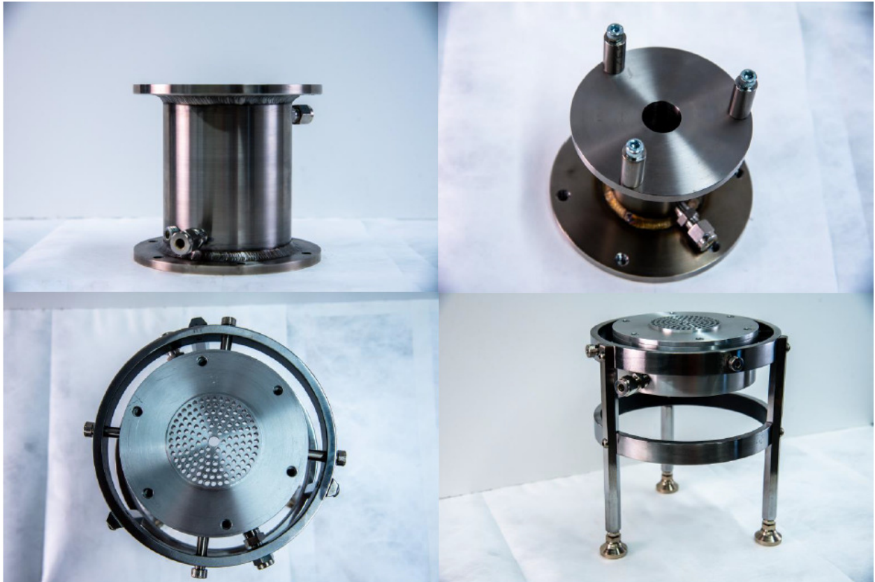
Figure 1.5: The four core parts of the burner are displayed. The top left image is the upstream plenum. The top right image shows where the quartz tube and flame will be anchored. The bottom left is the perforated plate located upstream the swirler. The bottom right is the burner stand with the with the perforated plate on top.
