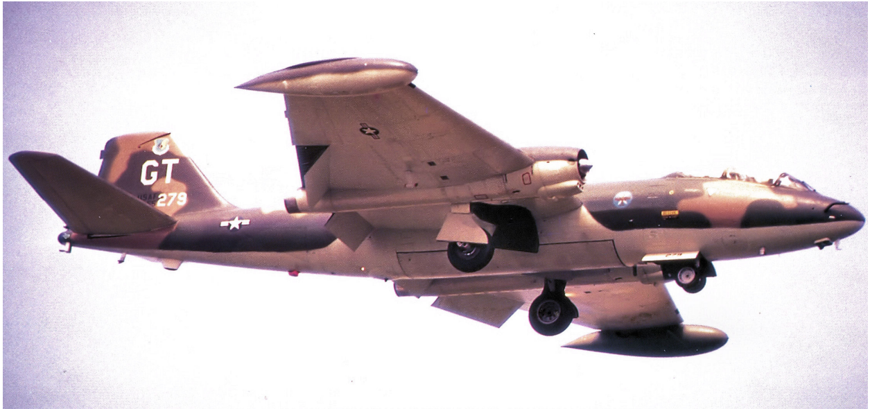
Figure 5: Glenn L. Martin Aircraft Company B-57 Bomber, this is the license built version of the British English Electric Canberra bomber [12].
