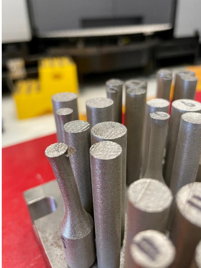
Figure 6.5 Photograph of Tensile Embedded with Shrapnel from Overheating.
