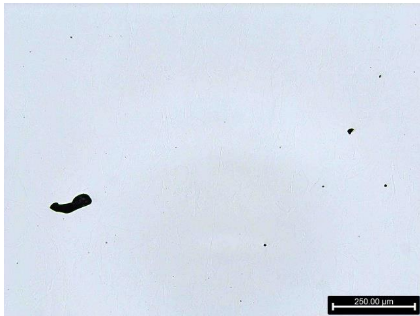
Figure 6.23 Defects from the Run #5 from Core1 XZ direction, 100x
