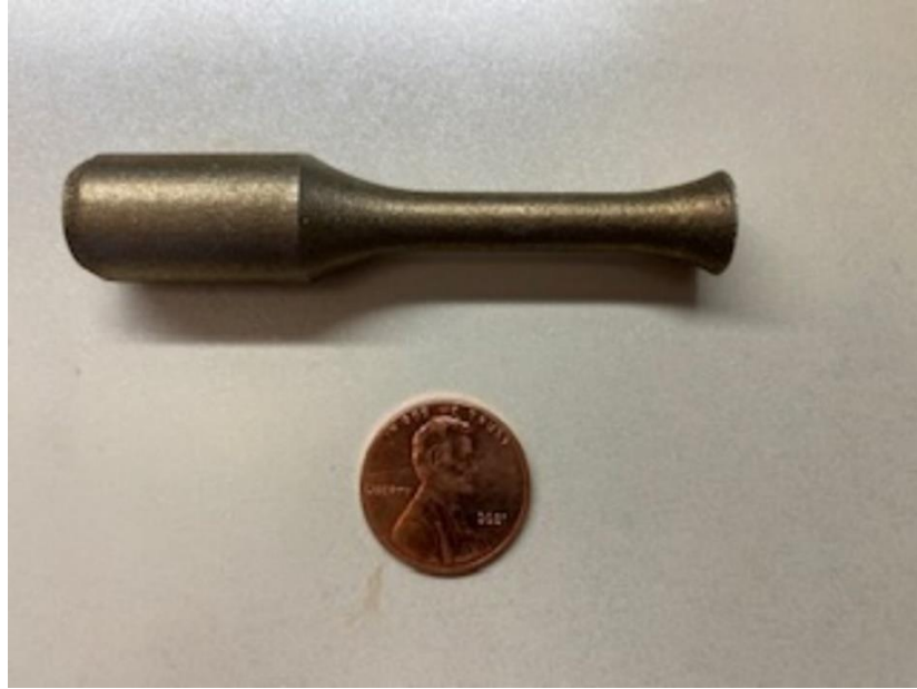
Figure 6.20 Sample configuration used for Metallographic sectioning
