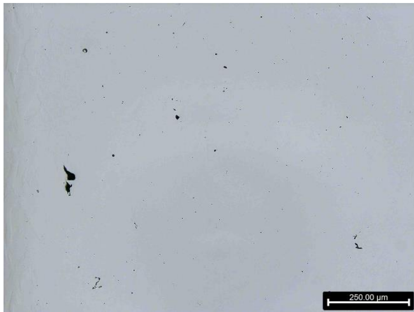
Figure 6.25 Defects From the Run #14 Core1 From XZ Direction, 100x
