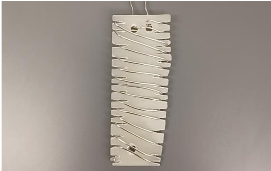
Figure 8.4: Example of test element holder implementing large gauge stainless steel wire for visual clarity.
