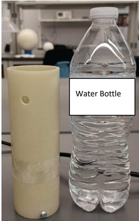
Figure 8.5: Constructed irradiation basket with 16 fl. oz. water bottle for scale.
