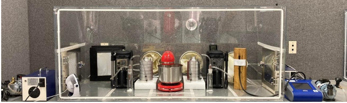
Figure 2.2 The system setup with two sets of samplers (Andersen impactor, AGI-30, and Bobcat).
