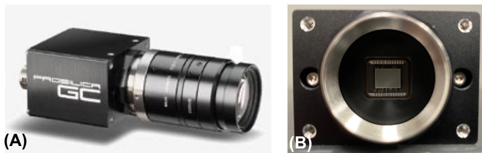
Figure 5.4: GC655 camera. (A): Zoom lens attachment. (B): CMOS sensor.
